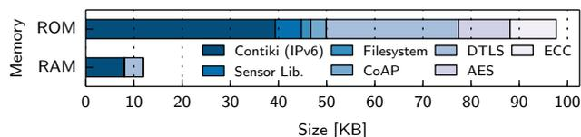
Figure 1. Memory requirements for a typical IoT stack.
